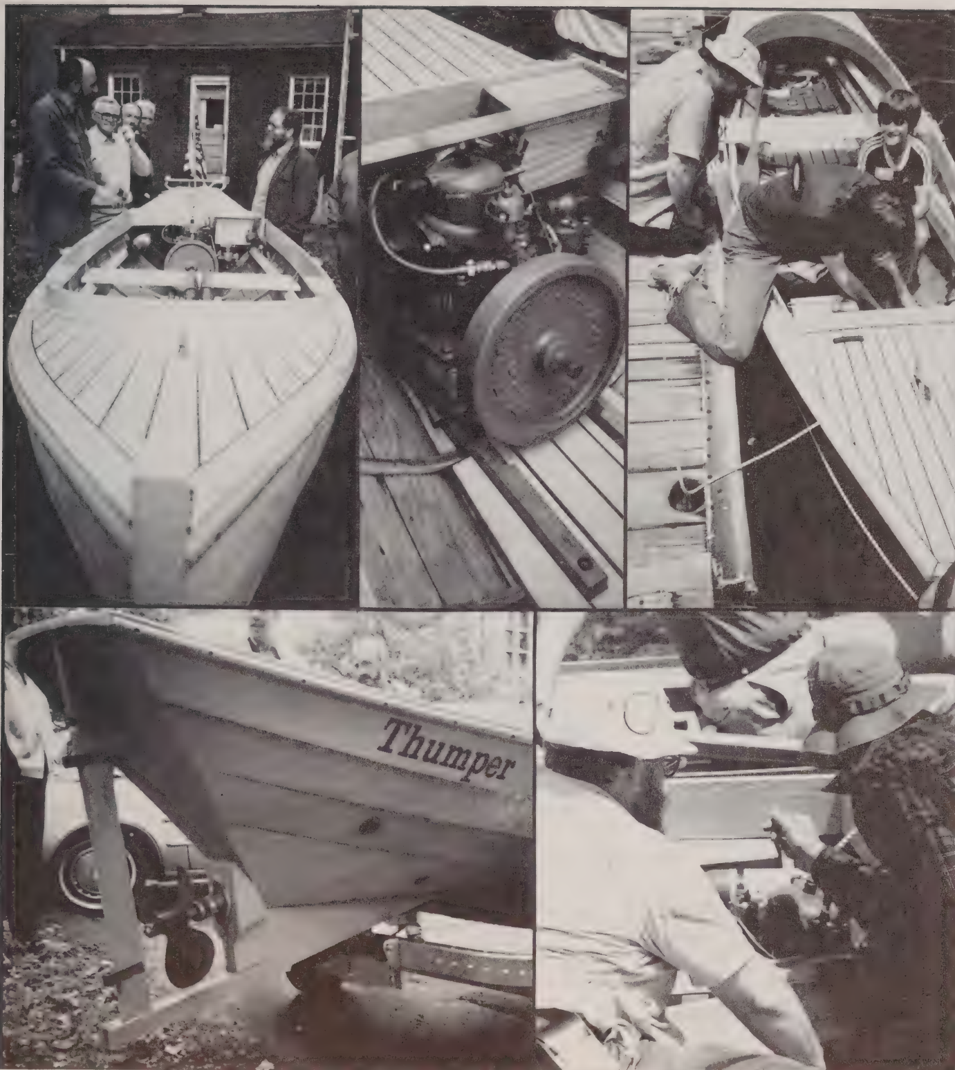
Across the top: THUMPER was on display at the June meeting of the Peabody Museum TSCA. The "thump" comes from here. Tinkering at Mystic. Across the bottom: Traditional dory transom, steeply angled propeller and shaft. Advice in progress.
