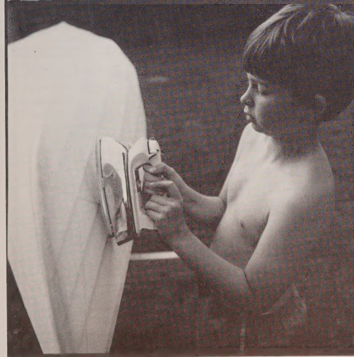
Chris at work on the SNOWSHOE. Framing up on the strongback and molds made from cardboard cartons. Stretching on the dacron and heat shrinking it tight. Off the molds, just cut them away. Finished out ready for painting. With dad, ready to head for the water.
