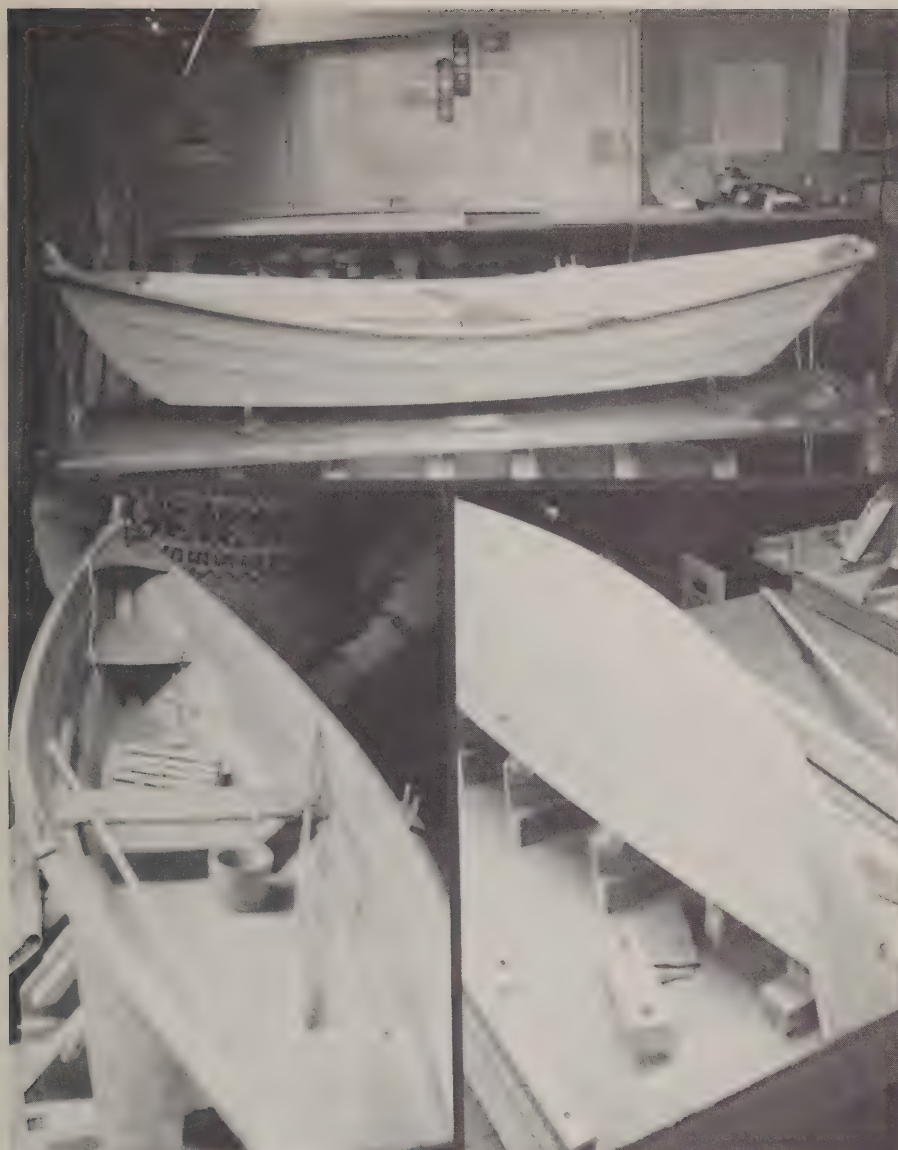
Top: A finished dory looks pretty real despite it's size. Bottom: All fitted out with its gear. On the molds, planking up just like the full size boat.
