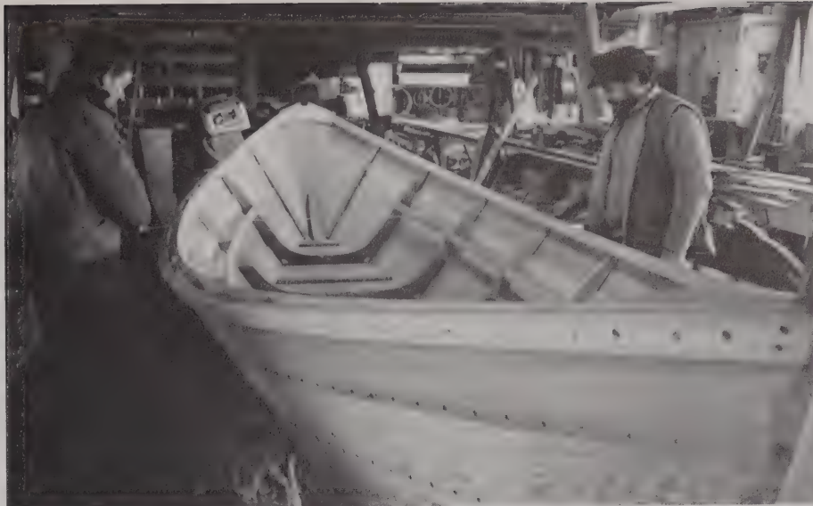
Ralph Johnson and Bob Elliott finishing off a 20' dory.
