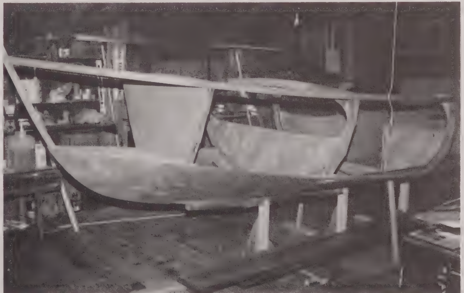
The building molds also form permanent bulkheads in the finished boat.
