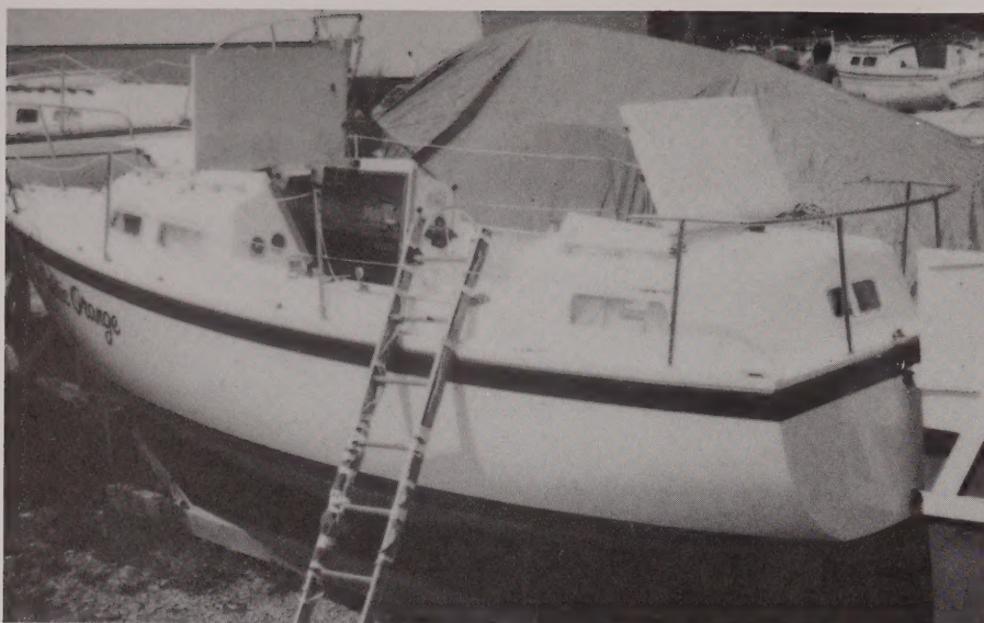
"Yeraz" as we first saw her at the yard. Note blade rudder in bracket; swing-up hatches, heavy and sturdy; instrument bezels port and starboard. She's on a low wooden cradle with keel retracted. This is what we fell in love with.
