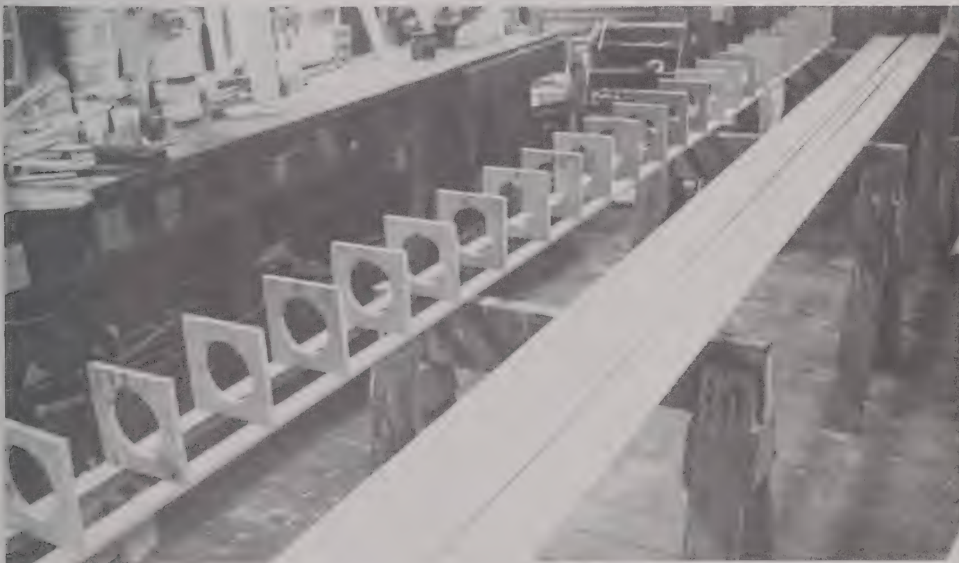
The very simple and inexpensive, yet effective, mast clamping fixture. It is ready to glue "Jolyon's" main mast. Those are the staves for it laid out on the saw horses.
