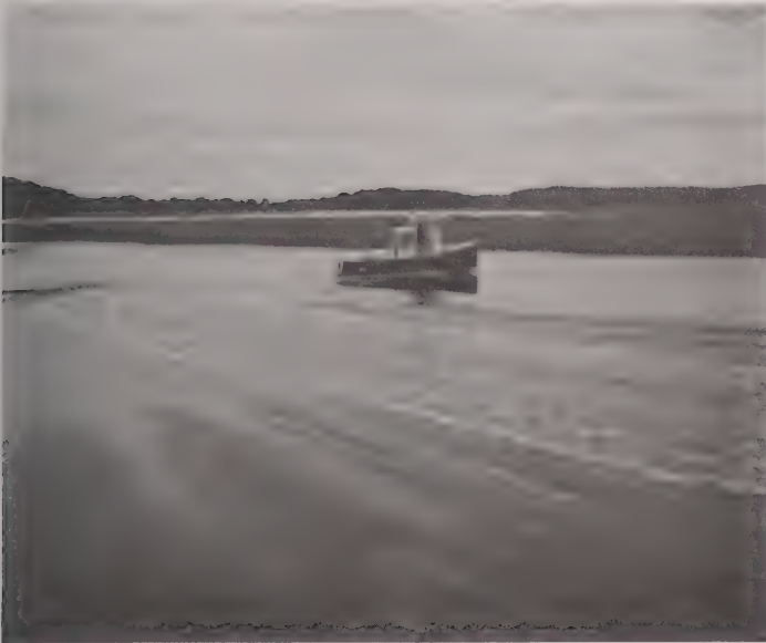
"Hawkeye" on the Jones River. The left hand column of photos shows the turn of speed with three aboard, skipper and two passengers at ease on the rear deck. Note how far up on a plane the boat is and the lack of lean in the turning position the boat assumes. The right hand column shows the boat with just skipper Montgomery aboard, the hull rises a little higher from the water onto a plane, but the speed was about the same by our admittedly crude calculations.
