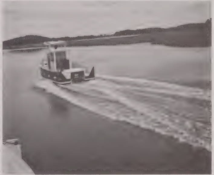
"Hawkeye" on the Jones River. The left hand column of photos shows the turn of speed with three aboard, skipper and two passengers at ease on the rear deck. Note how far up on a plane the boat is and the lack of lean in the turning position the boat assumes. The right hand column shows the boat with just skipper Montgomery aboard, the hull rises a little higher from the water onto a plane, but the speed was about the same by our admittedly crude calculations.
