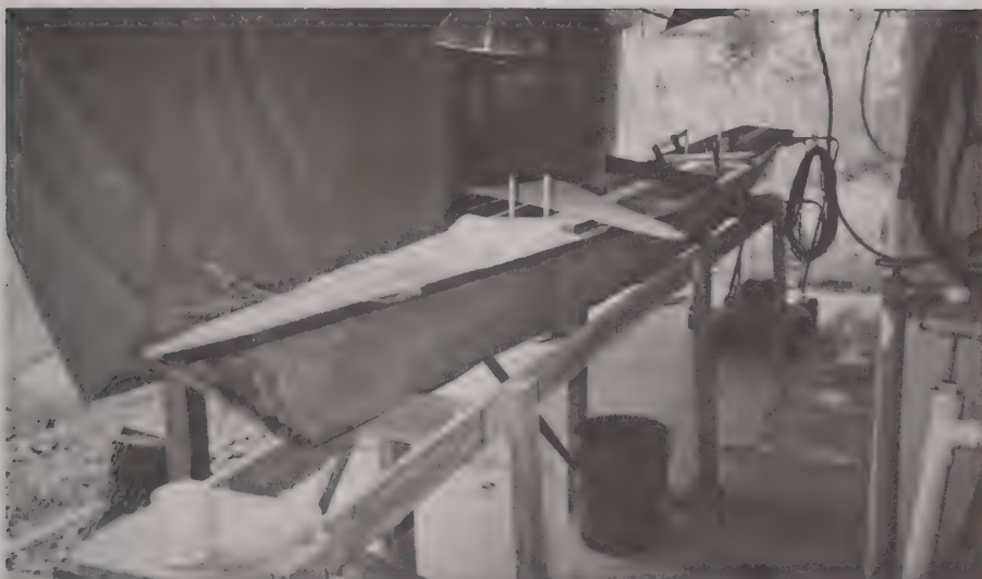
An ama under construction being filled with foam-in-place flotation.
