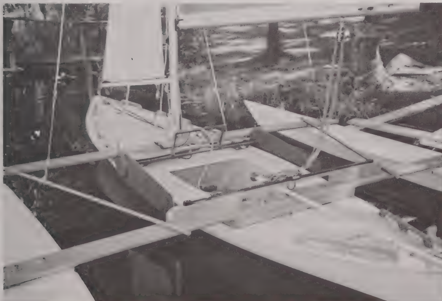
A look at the deck setup, note twin leeboard operating setup just behind mast.
