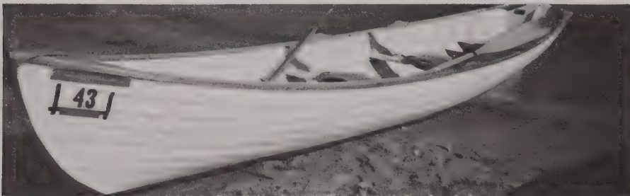
MODIFIED SEABRIGHT SKIFF LOA 17'8" LWL 15'0" BEAM 4'0" WEIGHT 145#
