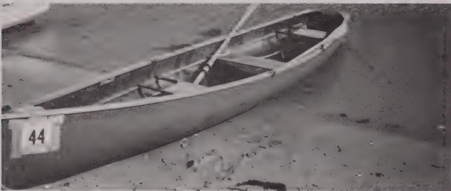
ADIRONDACK "GOODEOAT" LOA 17'0" LWL 16'0" BEAM 3'6" WEIGHT 114#
