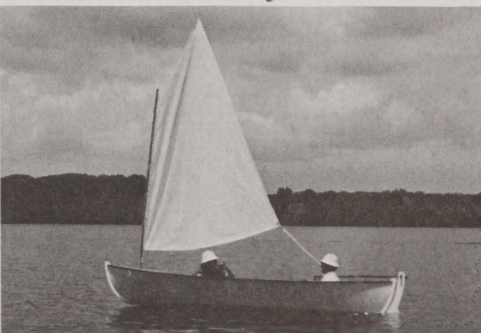
Matt Falcone brought his double ended skiff. Traditional lines hide the fact that the hull is foam cored glass.
