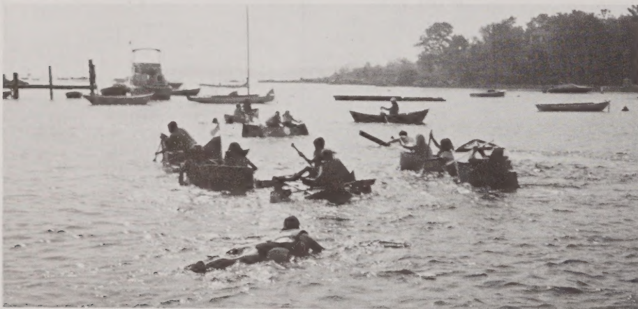
The girl chasing the pack "bottoms up" did not intend to go this way but her mockup jetski proved to have a very high center of gravity with little underbody and promptly turned turtle.
