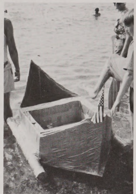
Cardboard tubes as flotation chambers were utilized on this other version of a "Silver Bullet, and on this pontoon boat concept. The latter held up very well, and was still happily out on the water when we left.
