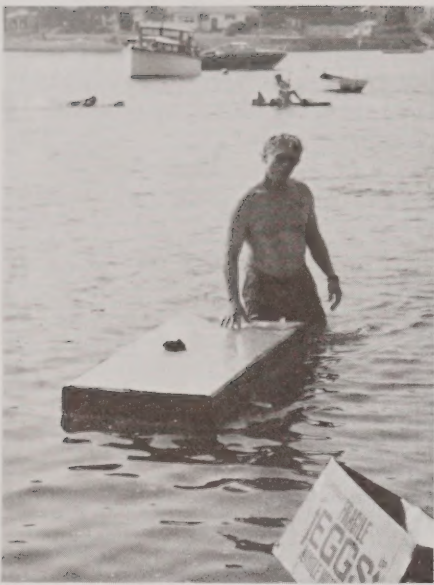
Basic watercraft, a flat carton, was fitted with a fin keel though. It was fairly stable but slow.
