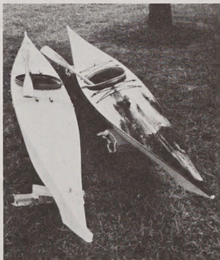
A pair of West Greenland style sea kayaks based on a build-it-yourself article in "Sea Kayaker" magazine. At left is Robert Sweeney's lashed wooden frame covered with sewn nylon skin. At right is Harry Mote's wood frame plywood skinned version.
