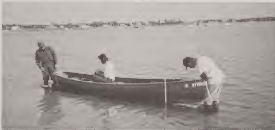
Waterline length is measured in this floating jig with an oarsman aboard.
