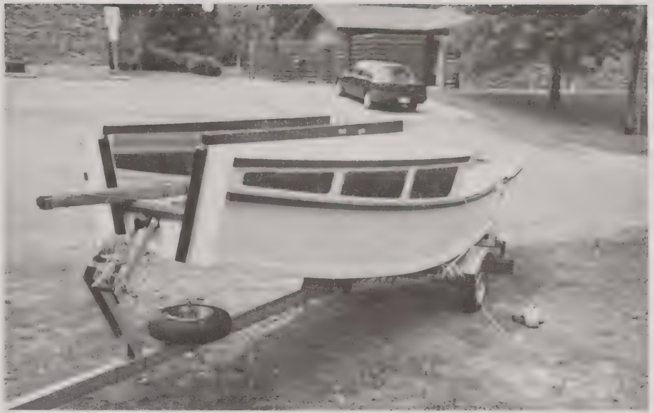
Front view of Pencilbox shows bow entry and cuddy walkway.
