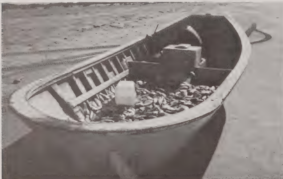
The catch fills the fish well, note construction details, with the inboard/outboard swung up forward of the well.
