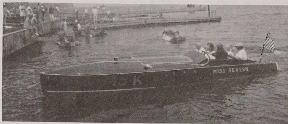
Miss Severn is a reproduction of a 26' Hacker Gold Cup racer owned by Gerald Davidson of Meredith, New Hampshire. She is powered by a V-12 1650 cubic inch Rolls Royce Merlin conversion done by Mark Mason of New England Boat & Motor.
