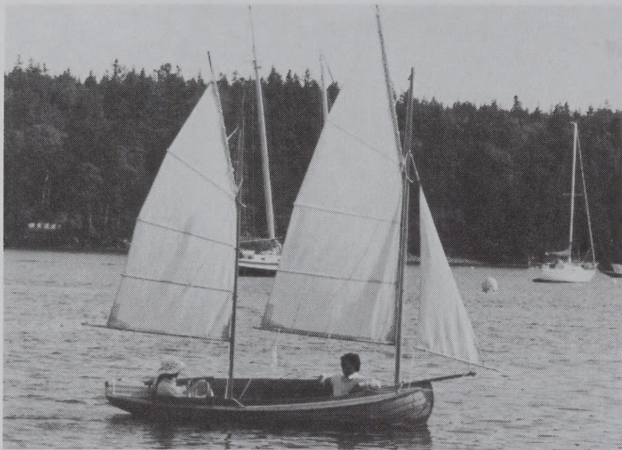
Thad Danielson (at the helm) built this elegant little 13' "Mini-Presto", a much scaled down version of Commodore Munroe's round bottomed sharpie concept. Thad builds totally traditional even to oiled finish and cotton sails. Redd's Pond Boatworks, 1 Norman St., Marblehead, MA 01945, (617) 631-3443.
