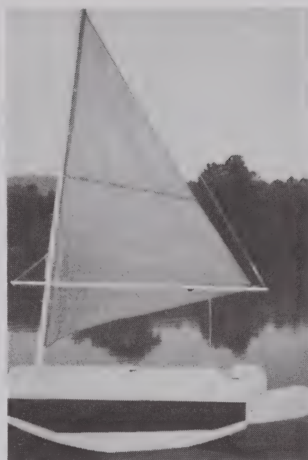
Rig with topping lift, vertical sheeting, single boom, no leech or vang reinforcement.
