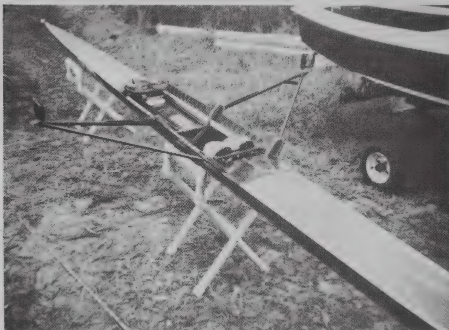
Lightweight racing single, carbon fiber hull, wood interior.
