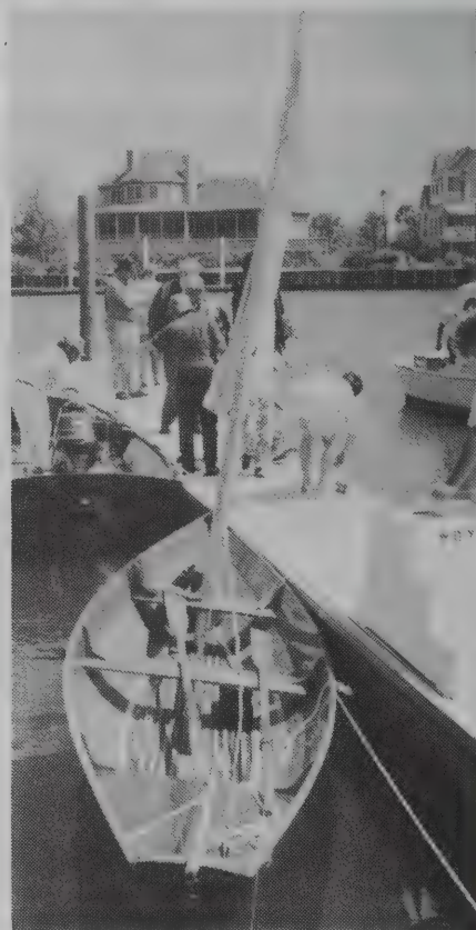
Swampscott Dory (one of four), plywood lap- strake construction, spritsail rig.
