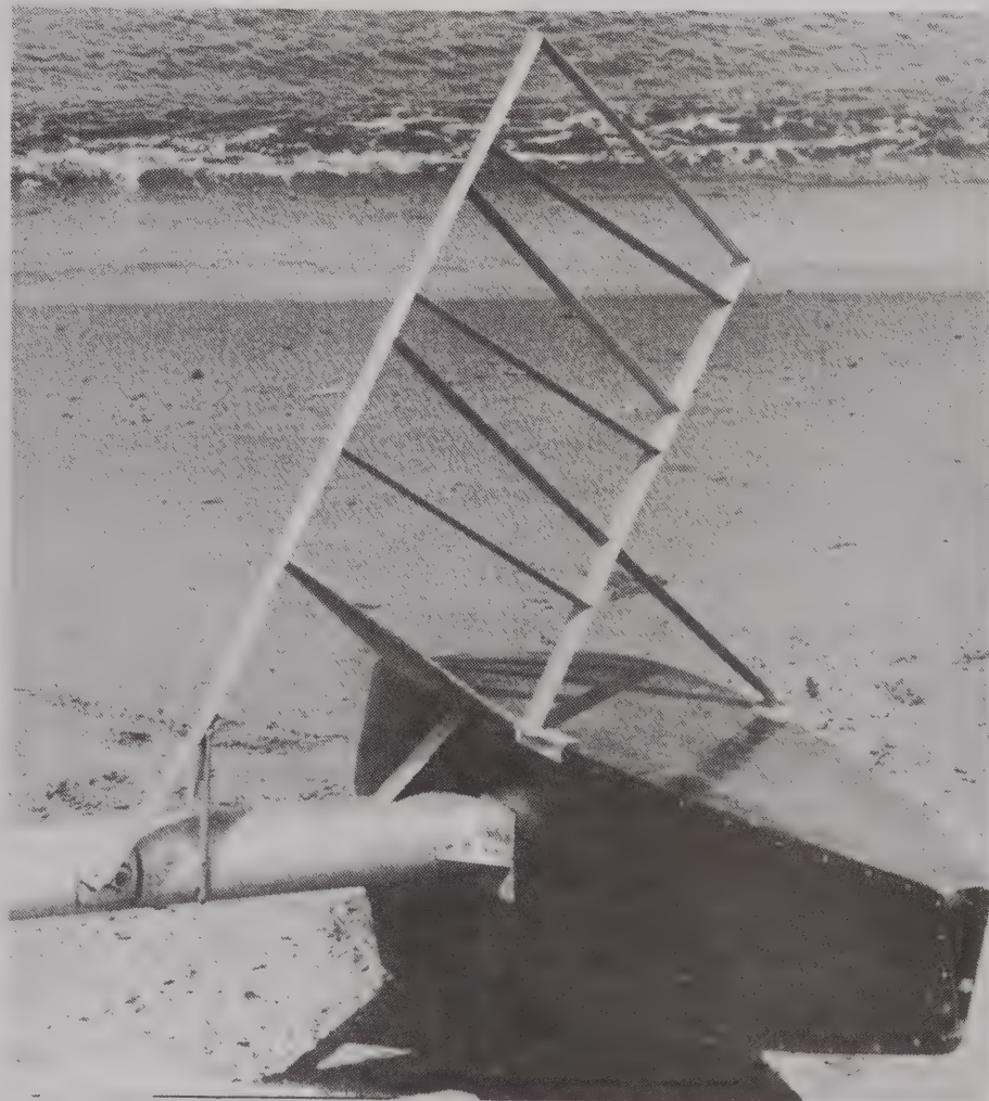
Detail of ama hydrofoil "ladder" in the "park" position.
