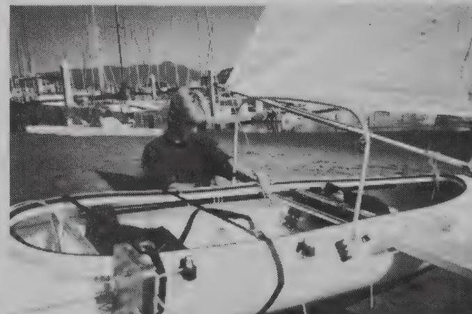
Rig details: Outboard mount, aluminum traveler and outrigger arm.
