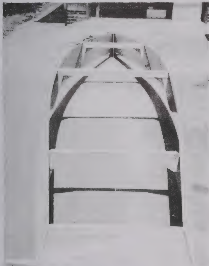
Checking hull symmetry with line from stem to center of transom. Line must touch centerline of all frames. Push hull around until it does.
