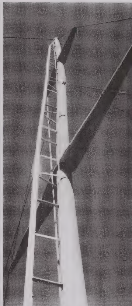
Above: The reinforced 4" PVC mast. Below left: The bowsprit rig. Below right: The mooring float, launching and hauling made easy with PVC rollers.
