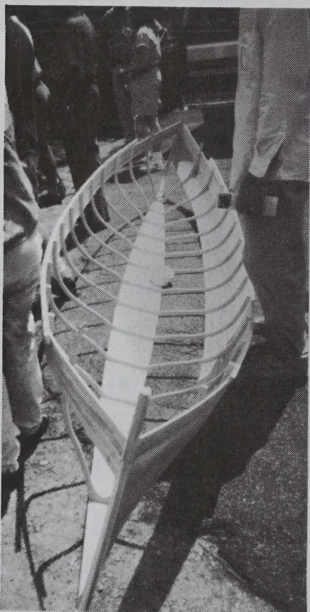
A partially constructed Adirondack Guideboat showing construction details by Steve Kaulback of Charlotte, VT.
