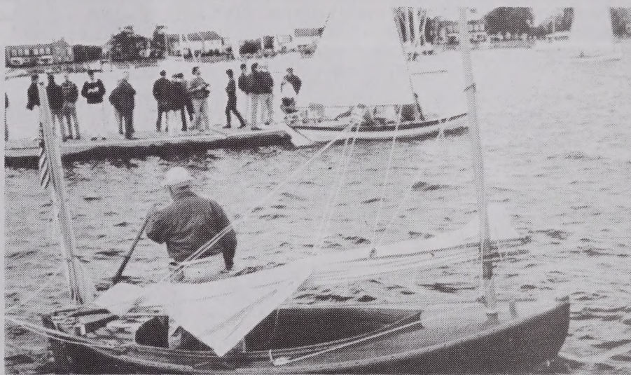
Sculling, a quiet, light and efficient auxiliary.
