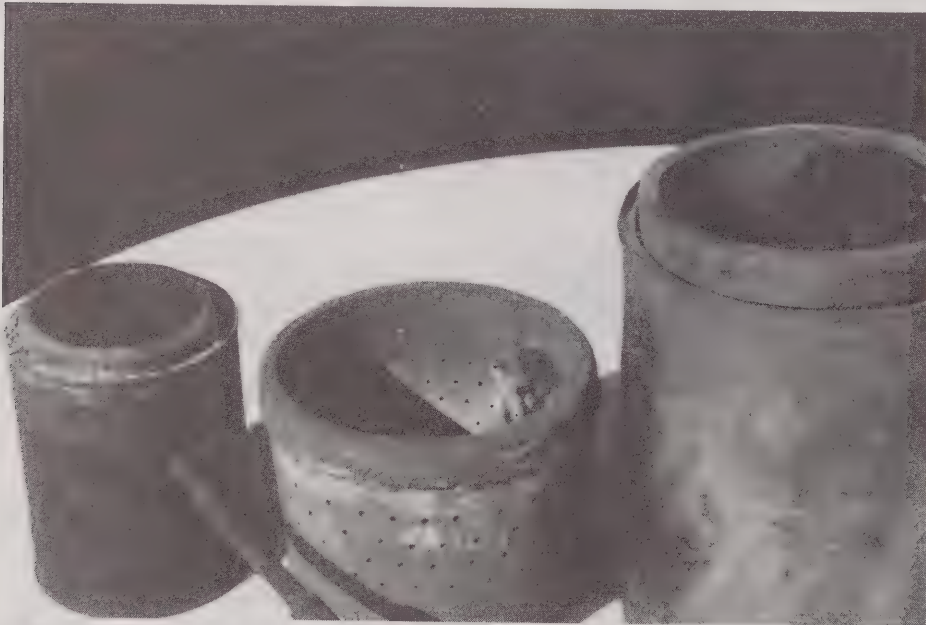
From left: The 1-qt. size burner; the pipe cap for the 1-gal. size with holes drilled; and the assembled 1-gal. size burner.
