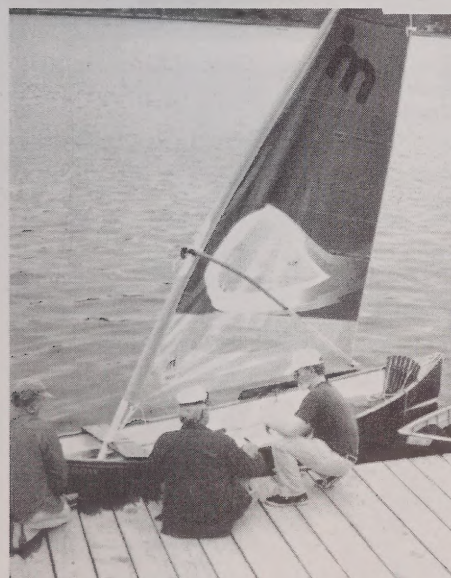
Chuck Raynor's one off C-flex Rangeley sported a radically raked aft windsurfer rig. Chuck pointed out this moved the center of effort far enough aft so he could sit in the stern and steer.
