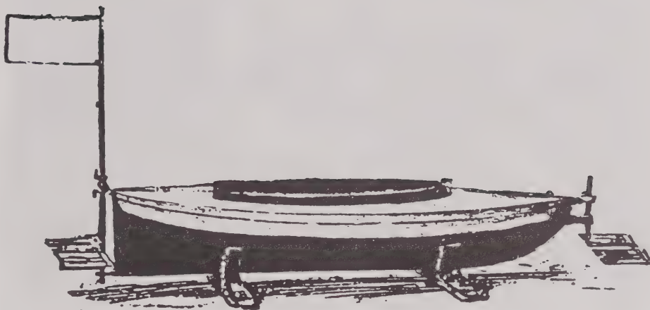
A drawing of the Autonaut showing the arrangement of fins and steering flag.
