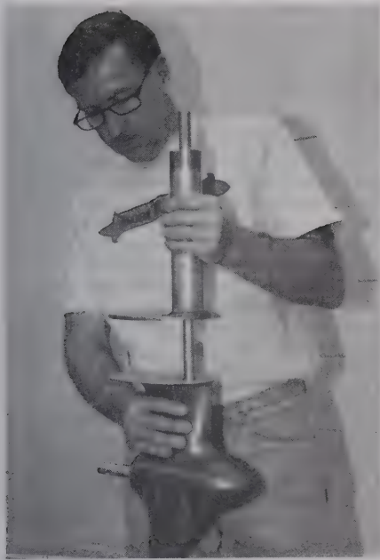
The pipe/flange assembly bolts atop the flattened cavitation plate of the outboard lower unit.
