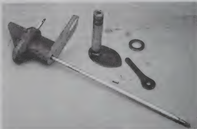
These are the metal parts that are cut to shape from steel from the patterned parts. The central sub-assembly is a pipe welded to a flange that in turn will bolt to the lower unit drive shaft. The tiller arm, to the right, will bolt atop the pipe/flange assembly.
