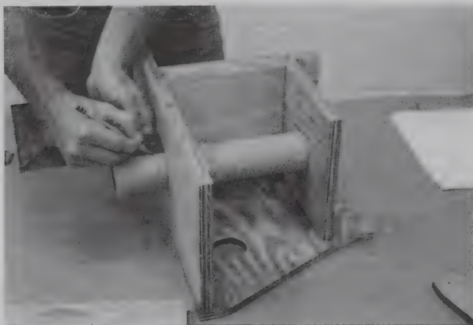
A fiberglass tube, made over a pipe mandrel, is epoxied to the wooden mount.
