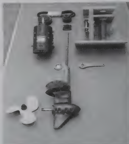
The various components of ED; belts, pulleys, assembled plywood mount with fiberglass tube, bearing collars, tiller arm, pipe/flange assembly, prop, and a portion of an outboard lower unit.
