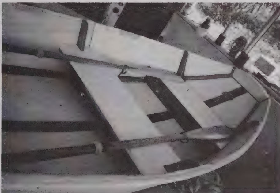
Auray punt (Bolger/Payson) prefab kit, mailed to Culebra, Puerto Rico. Put together, brown strip down center bottom epoxy, tape seam, chines epoxy/fillite/silica powder.
