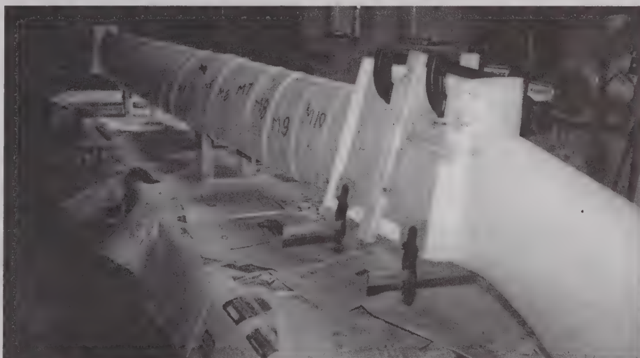
Foam rubber wrap presses fiberglass tightly to the mold surface.
