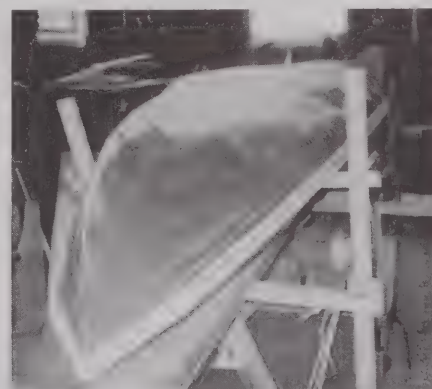
21) The canoe is now turned bottom up and supported with upright and cross pieces clamped to the wings.
