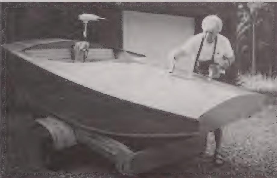
Fiberglass top and bottom and with best marine paint.
