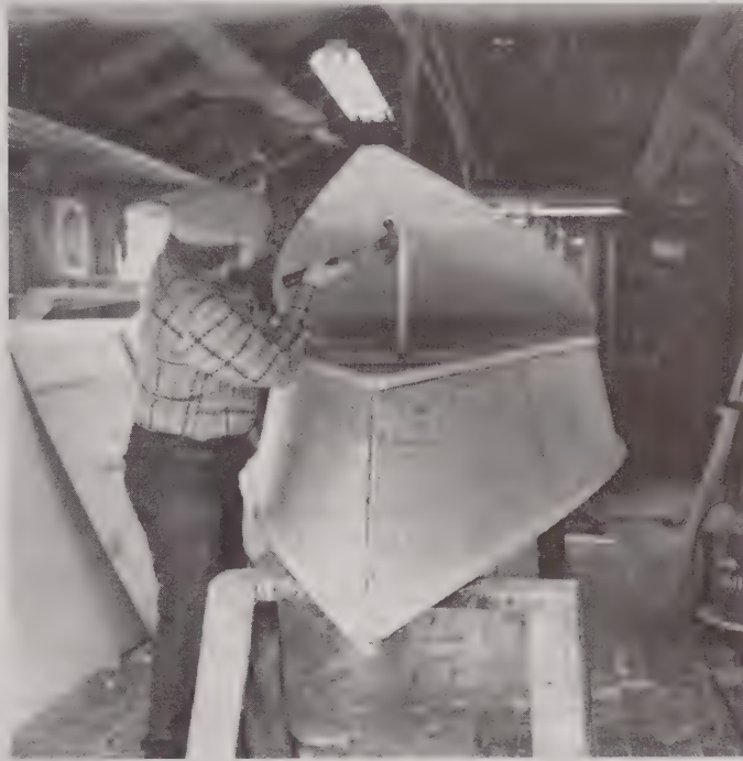
Bottom is fitted piecrust fashion and butt jointed fore and aft.
