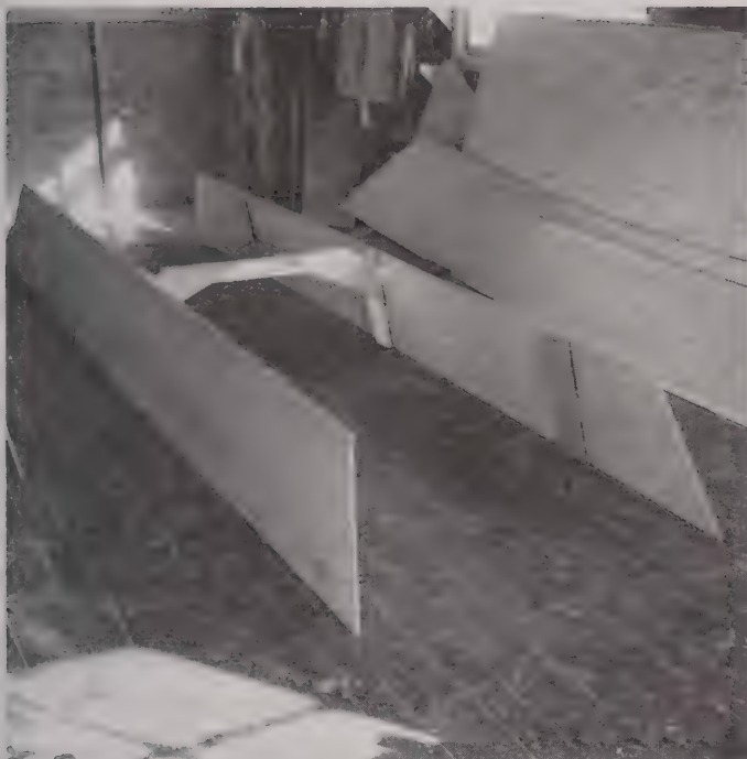
Buttstrapped sides are fastened to midframe.
