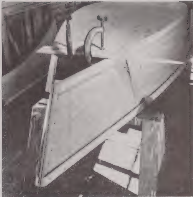
Bottom is fitted piecrust fashion and butt jointed fore and aft.
