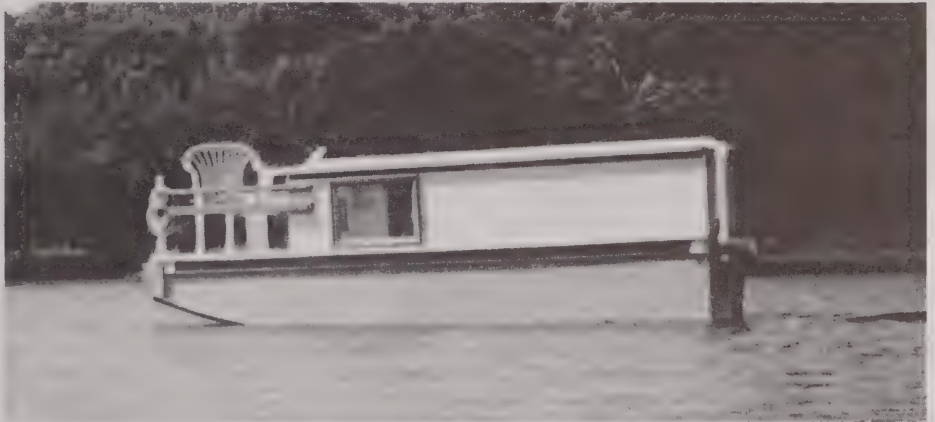
A side view of the Harmonica-class shanty boat. Two plastic lawn chairs sit on the bow, the railings are ball-and-post, taken from a Victorian porch roof design.
