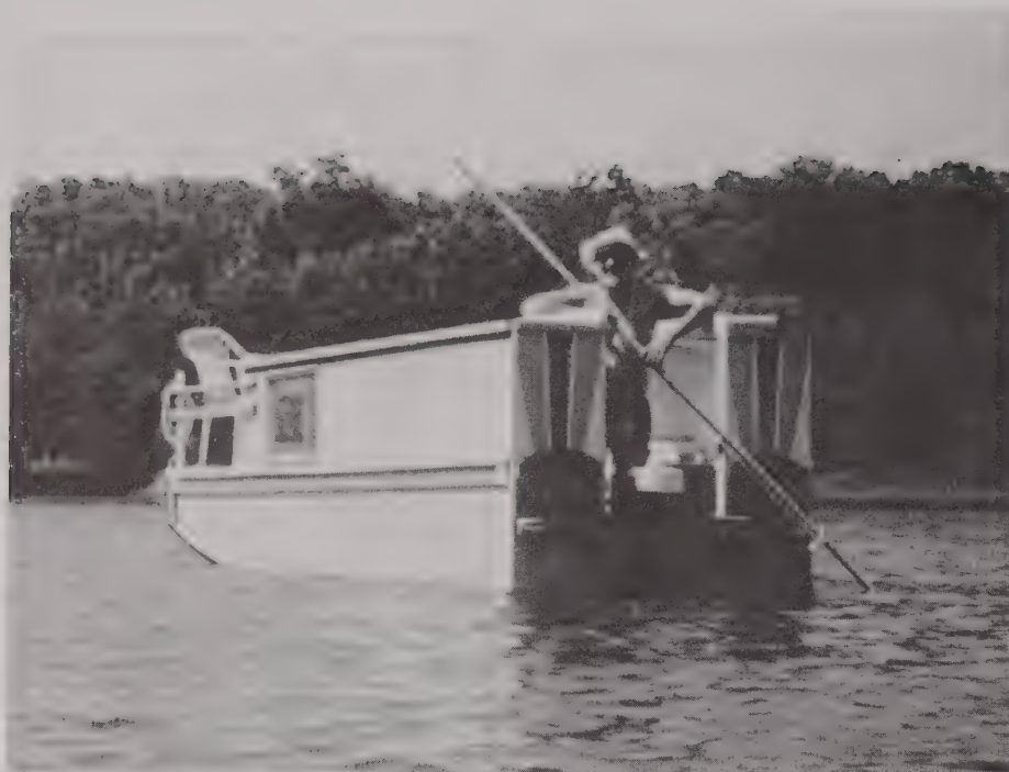
A stern view of the boat, David Unruh aboard with a bamboo quont. The bamboo is used to pole the boat around, and doubles as an emergency paddle, which works well even without a blade. The sunburst on the stern is part of the (still emerging) Victorian decoration.
