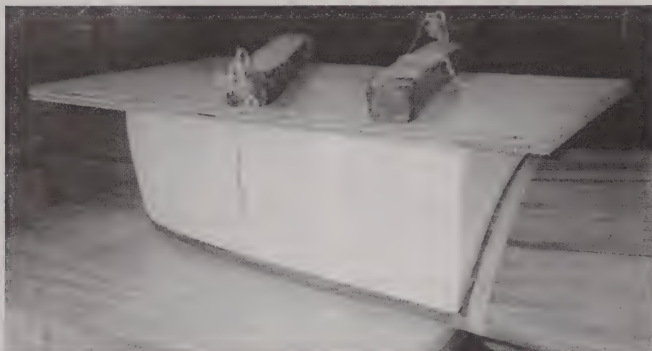
Gluing down foam block for stern.
