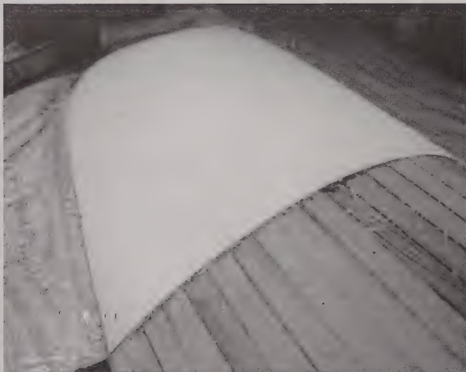
Foam end — shaping with surfboards.
