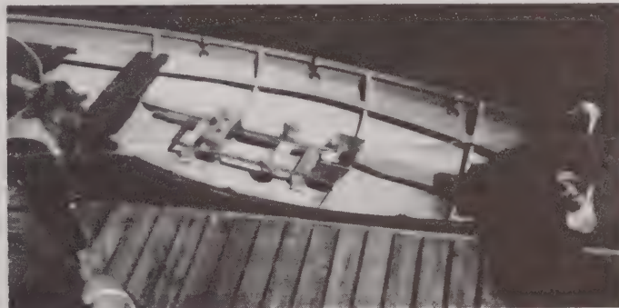
Sliding Seat: Feet fixed, seat moves with oarlocks.
