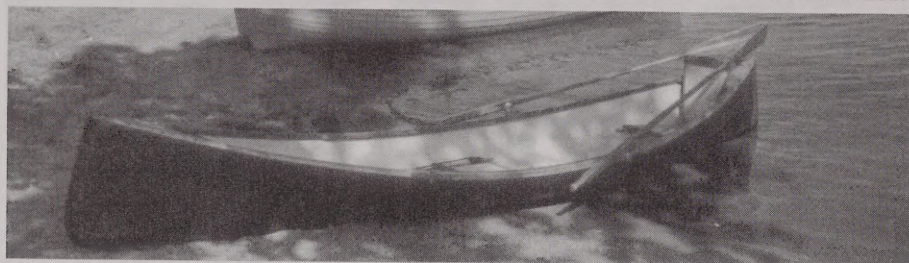
Adirondack Guideboat built by Steve Kaulback in 1997, composite construction (read Kevlar). Painted traditionally, "I don't build no gold colored boats."
