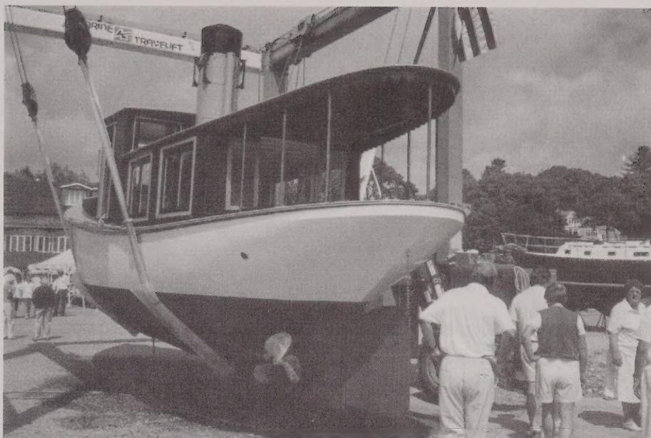
Pre-launch look at the underbody, narrow and sleek, lots of deadrise, classic old low-powered hull design.
