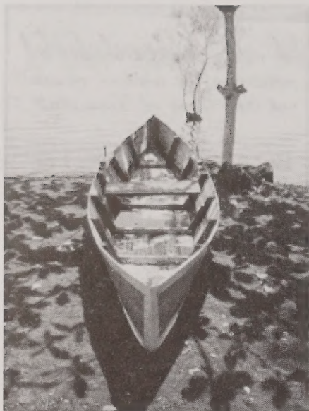
Catemarco skiff. Note thole pins, really guideboat type pivots, and bottom planking.
