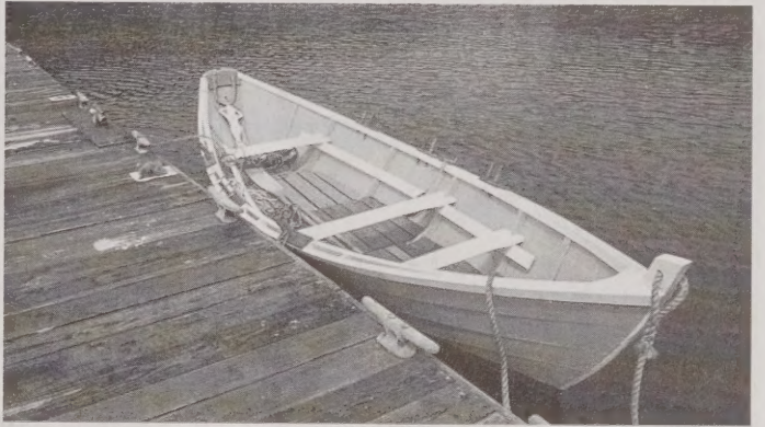
Scott Malvitch of Corvallis built this Banks dory in the traditional way, out of oak and Port Orford cedar.
