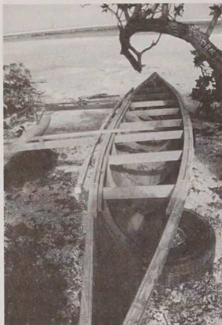
The hull is symmetrical, but the outrigger is curved more towards the hull side.
