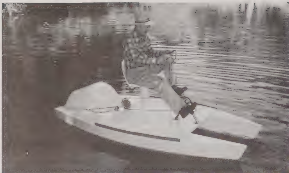
The Pedal-It is a 9'4" asymmetrical catamaran propelled by a bicycle pedal and sprocket chain driven to a paddlewheel.
