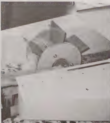
The paddlewheel, made from plywood, rotates on a shaft between the two hulls.
