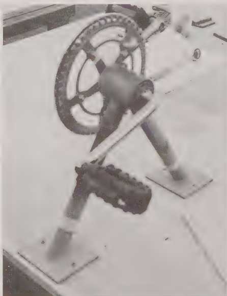
The bicycle pedal/sprocket is salvaged from a second hand bicycle, and is inverted and mounted on the bridge deck spanning the pontoons. The seat raises, tilts, pivots, and moves fore and aft to suit the comfort of the peddler.
