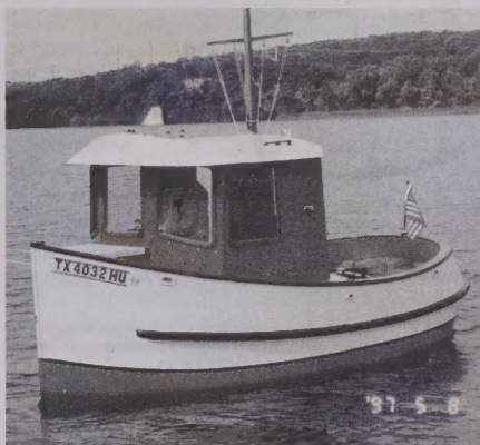
Tony's "Tug-A-Lug" , LOA 15'3", beam, 7'4", hdrm 6', draft 20". Powered by GE 10hp 36v electric reversible motor w/solid state controller. 36v onboard automatic battery charger w/25' 110v short recharge cable. Attractive large teak ship's wheel. Compass, 36v ammeter, voltmeter, twin horns. Ignition switch & throttle controls on the console. Separate 12v battery electrical system. Dock lines & anchor w/100' line. Large solid brass ship's bell. 2 fwd cabin windows open for ventilation. 20" x 24" fwd hatch. Cabin door fitted w/porthole & security lock. Fire extinguisher. Large formica countertop in cabin & folding formica-top table in cockpit. Lots of storage bins in cabin. Removable white bimini summer top over aft cockpit. Folding wood mast w/cross arm; flag lines. Approx weight 1250lbs, on new custom-built Magnum trlr totals 2070lbs. Loads & off-loads easily, tows nicely. Easily carries 2-6 people & handles well on local lakes. Slow but very maneuverable. Clear title. This crowd pleaser is an environmental jewel, no fumes, no noise, no fuel, no pollution. Just quiet, leisurely pleasure boating. $12,750. MORINE BINGELIS, 8509 Greenflint Ln., Austin, TX 78759, (512) 345-1537. (11)
