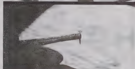
How nails are picked up and held by grooved tweezers.
