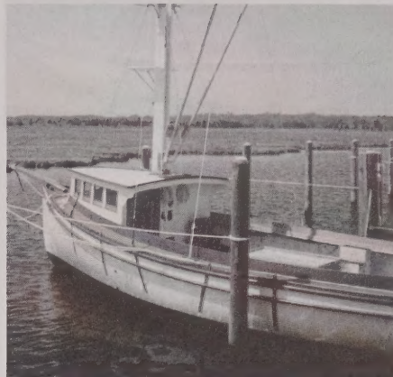
'83 Marshall Catboat Hull , 26' x 12' x 2'6". FG is about 7/8" thick at keel, solid, no core. Finished out by Concordia Yachts, S. Dartmouth, MA. Chosen for its stability for a man in a wheelchair. 75hp, 4cyl FWC Volvo diesel, 2:1 reduction w/less than 100 hrs. Edison hydraulic steering & wheel. Twin bilge keels. 2 bronze sea cocks are only holes in bottom of boat. 5 dbl bronze steps on rudder & hull, 4 10" & 1 12" cleats, 4 chocks, 12 HD chainplates for any combo, dbl rubrails w/1/2 rmd guard, all above hvy bronze. Cabin section about 1" of insulation, 9 cabin windows all opening, molded in deck shelf entire hull length, full length engine stringers 2" x 10", extra stiffeners in hull. Crows nest, 2 gin poles. Gear that goes w/boat too much to list or remember. Also scale model of boat incl. $25,000. '72 Marshall 22 , new sail & sail cover '99. 22hp Palmer (gas) runs vy well. Larger sail area than normal. Open arrangement below. Nds cosmetics & repairs around deck icebox. Sailed every day from May to November weather permitting. $19,000.
