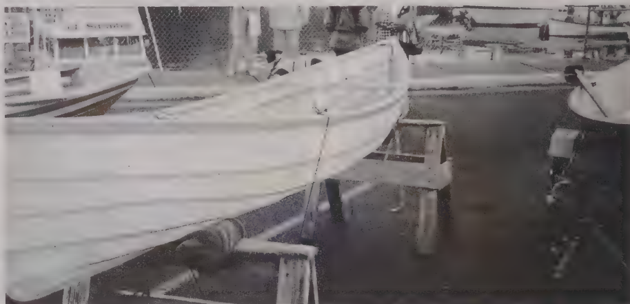
14' Platt Monfort geodesic aerolite canoe built by Marty Vukonich of Otis, Oregon.
