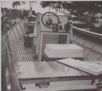
18' center console skiff built during the first boat building class at the Lake Pontchartrain Basin Maritime Museum.
