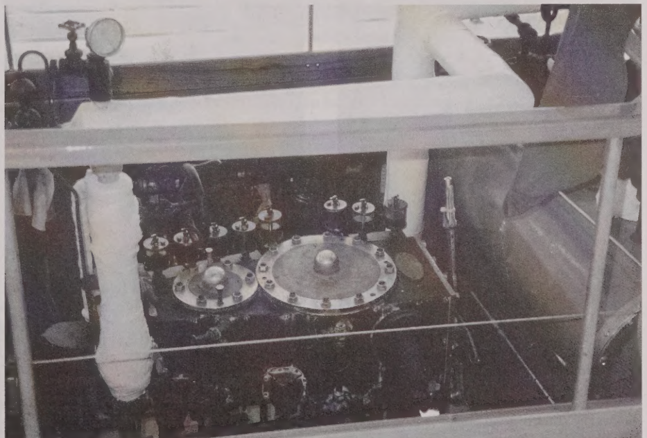
The 40' Steamboat Mascot attracted a good deal of attention. Mascot was built in 1997. The engine, a 1918, two-cylinder, 50hp compound steam engine from a USN yard tug which operated in Baltimore, pushes Mascot at 7 knots, running on steam pressure of 160 200psi turning a 38" propeller at 180rpm.
