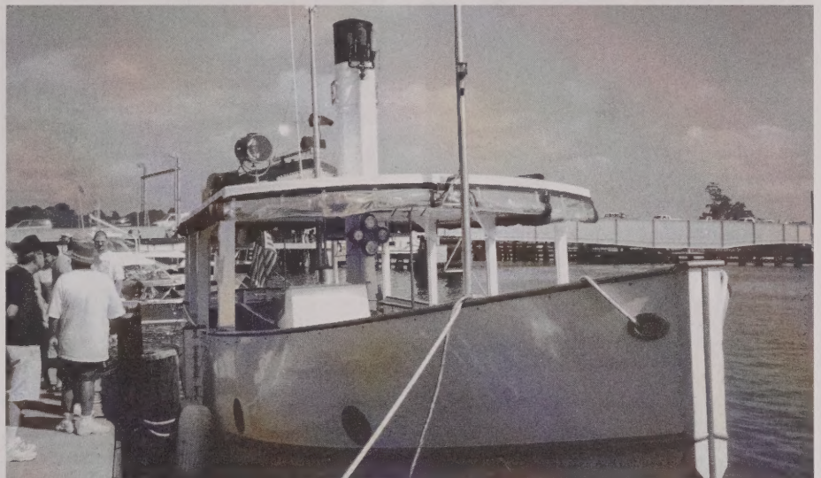
The 40' Steamboat Mascot attracted a good deal of attention. Mascot was built in 1997. The engine, a 1918, two-cylinder, 50hp compound steam engine from a USN yard tug which operated in Baltimore, pushes Mascot at 7 knots, running on steam pressure of 160 200psi turning a 38" propeller at 180rpm.
