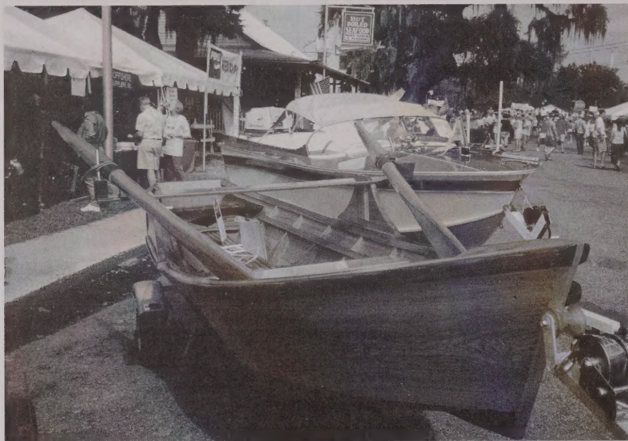
A bright finished rowing skiff with lots of rocker and what appears to be a stand-up rowing setup, note the height of the oarlocks.
