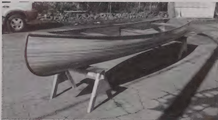
Trout Boat, stripper construction.
