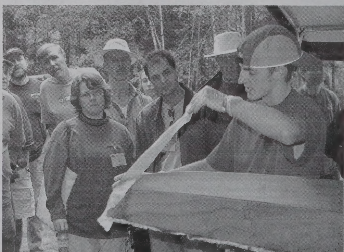
Travis soule demystifies application of fiberglass cloth to a stitch and glue hull.
