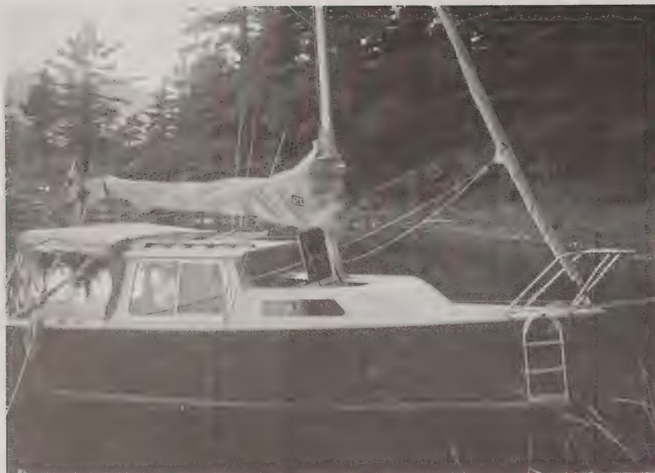
Return to Forever tucked into nook, North Channel of Lake Huron. Note raised fiberglassed galley section with fixed windows and dodger over cockpit.
