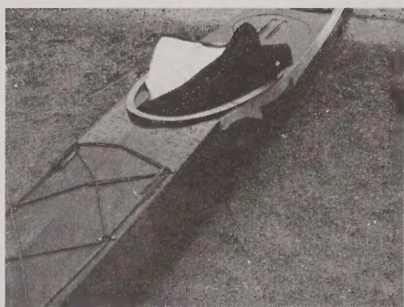
The "puzzleboat", an unusually veneered Guillemot stripper kayak.
